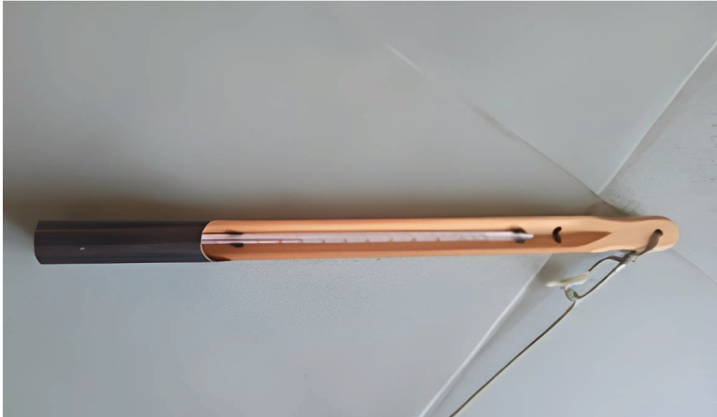
Gambar 3. Armored Case Assembly
