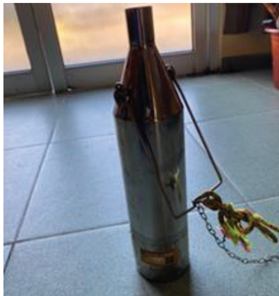
Gambar 6. Beaker Sampling Tool
