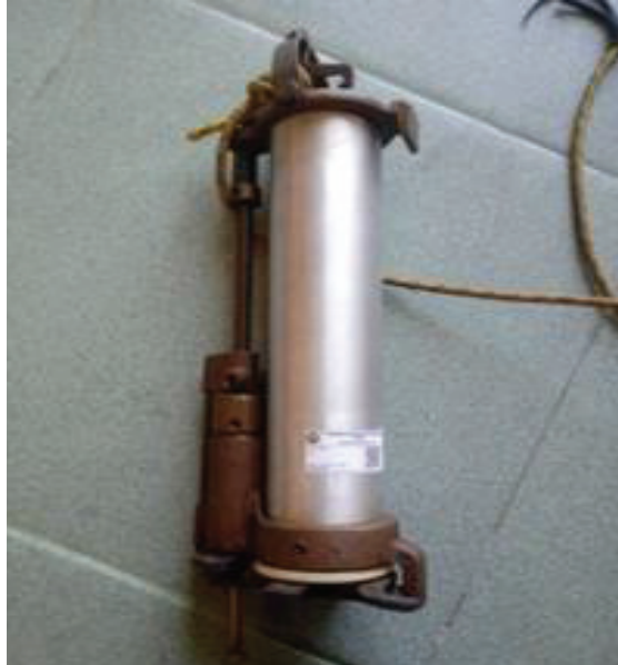
Gambar 5. Core Thief Sampling Tool
