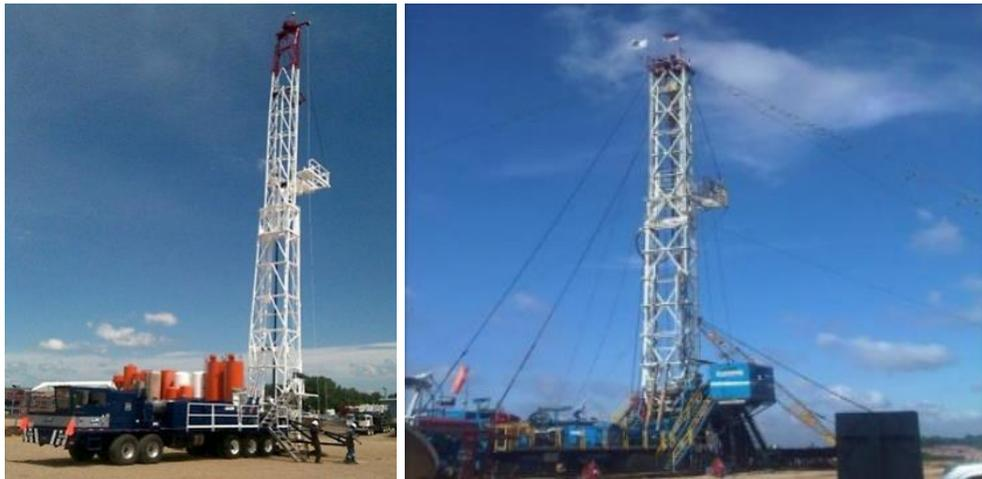
Gambar 3. *Vertically Telescopic Mast* dan *Guyed Telescopic Mast*.
