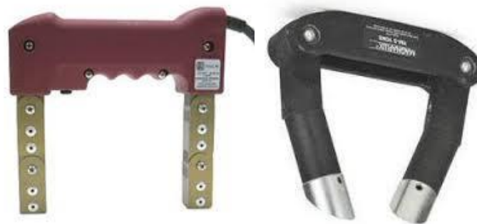
Gambar 5. Yoke (a) Yoke elektromagnet; (b) Yoke permanen.
