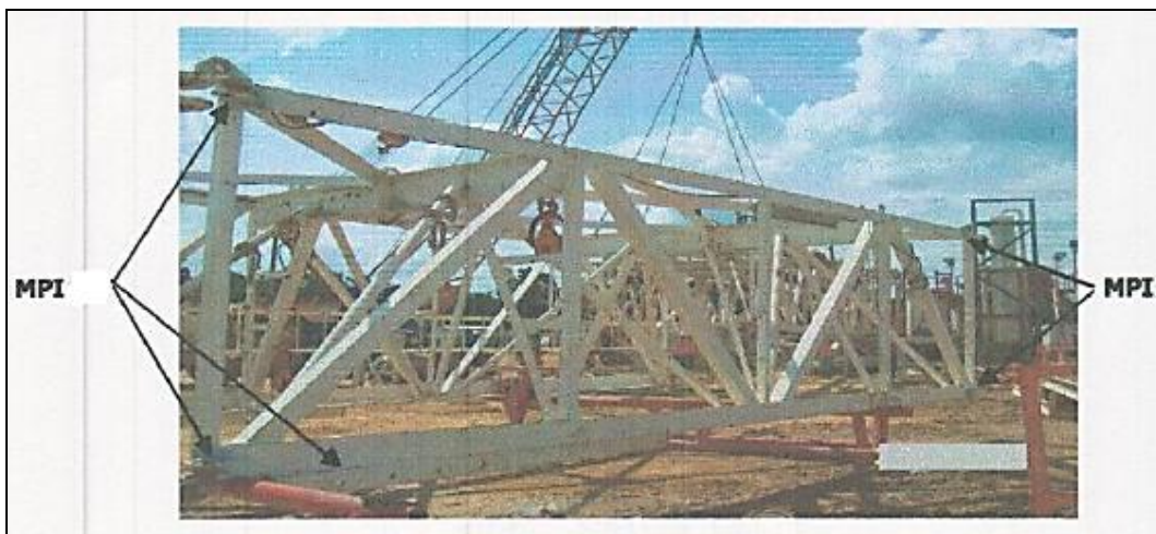
Gambar 11. Contoh monkey board padeye dan middle mast legs .
