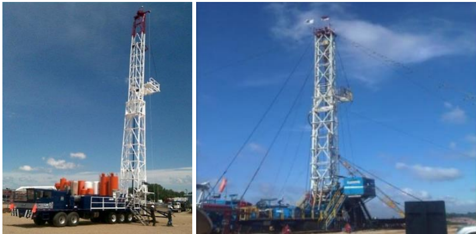
Gambar 3. Vertically Telescopic Mast dan Guyed Telescopic Mast.
