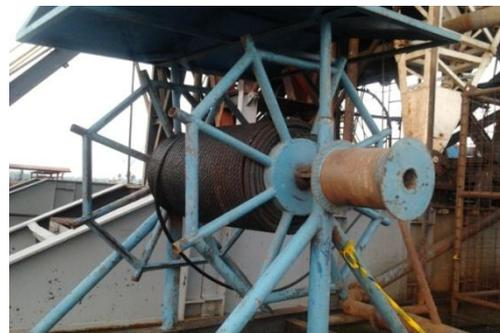
Gambar 8. Drilling Line Lubricator dan Drilling line di Reel
