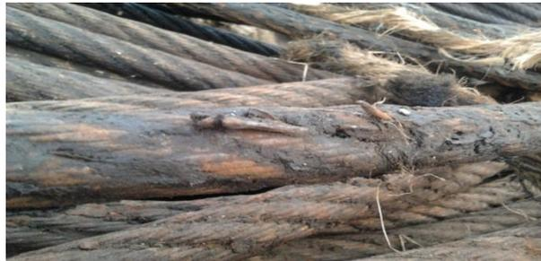
Gambar 7. Contoh Drilling Line Yang Rusak
