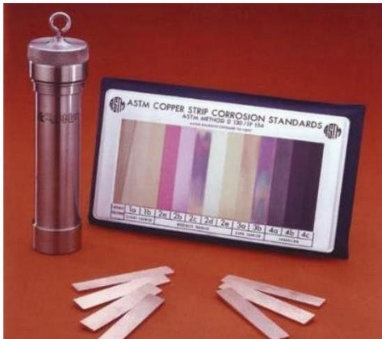
Gambar 7. Copper Strip Corrosion Standard
